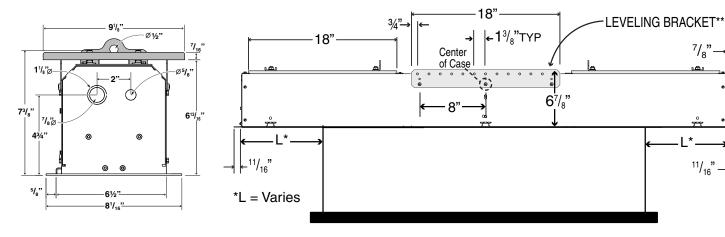
For ceiling cutout subtract 11/2" from case length and width (measured from outer edge of flanges).
